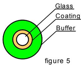
A thermoplastic material is extruded directly over the acrylate coating, increasing the outside diameter of the fibre to 900 micron (0.9 mm), an industry standard. (figure 5)
